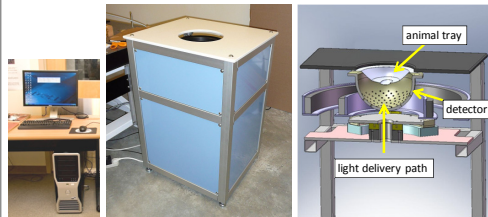
(left) acquisition/reconstruction console, (middle) scanner cabinet, and (right) diagram illustrating light delivery, animal tray, and detector position
